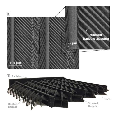
Barbules as connecting elements between feathers. (a) Their spacing is measured as the distance between barbules. (b) An additively manufactured bioinspired model demonstrates the orientation of the barbule membrane flaps between barbules.
